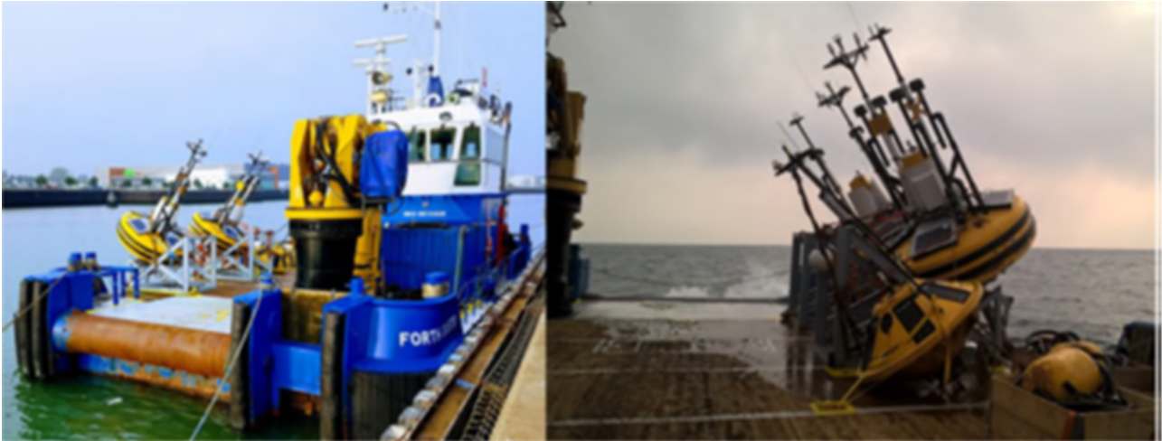
Figure 2.7. FLS secured on the deck of vessel.
