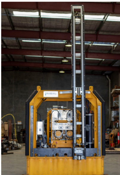
Figure 2.9. Seabed CPT unit with needle probe outboard mast on frame (left) and needle probe (right)
