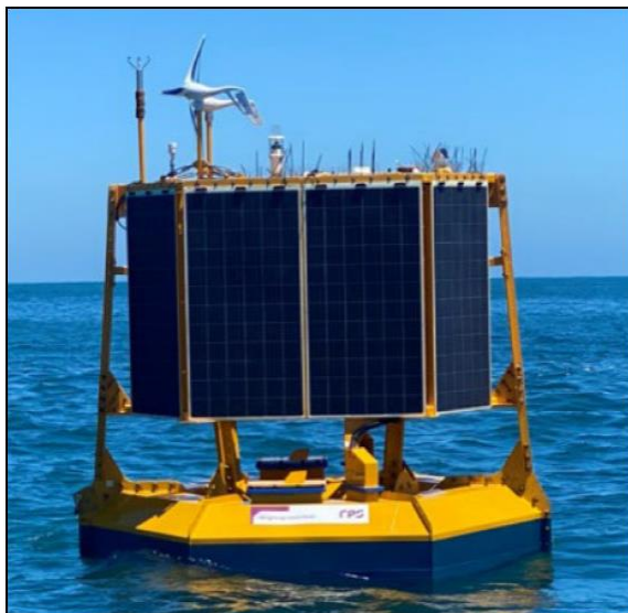
Figure 2-2 RPS LiDAR 3.5 Buoy (Source: RPS, 2024a)
